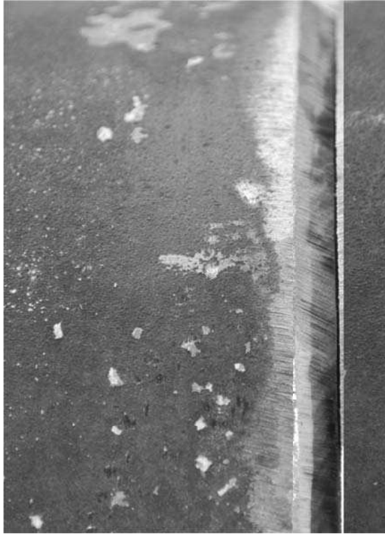
Typical fit-up using a 45 degree Single Bevel.
